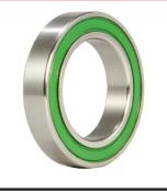
Our XD-15 Pro bearing utilizes the same XD-15 steel as our Xd-15 Corsa bearing, only different in design. XD-15 Pro bearings are 15° angular contact sealed cartridge bearings. The bearing raceways are deep-groove to improve longevity and increase ball size. XD-15 Pro bearings use Grade 3 Silicon Nitride ceramic balls and are sealed on both sides using LLB Nitrile seals. These bearings are available in 24mm AND 30mm ID for most of our bottom bracket solutuons.
