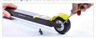
06. The new bolts which come with the wheel set must be used in order to ensure safety when using the rollerskis. Apply some threadlocker to the thread before fastening the bolts. Bear in mind that the adhesive has to dry for 24 hours before the rollerskis can be used.
